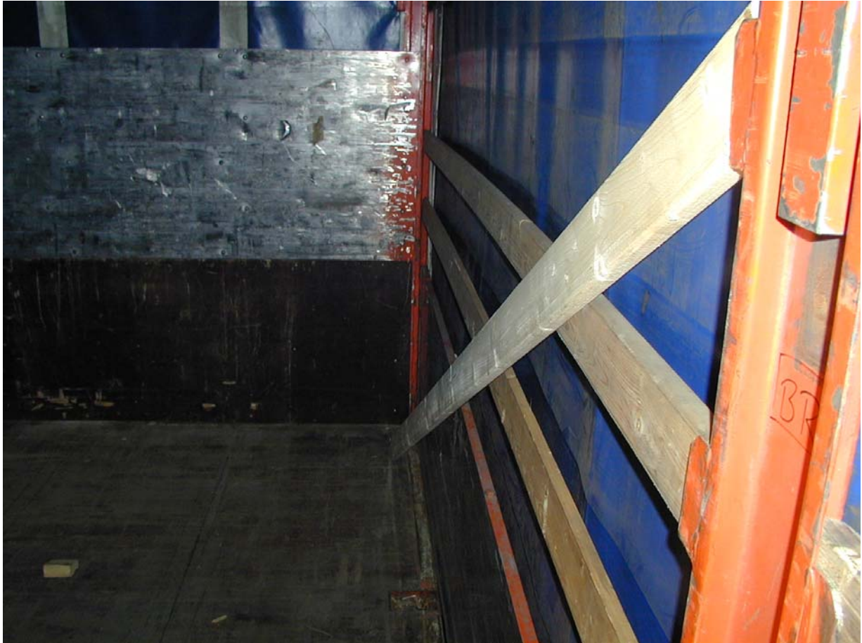
Figure 14: Wooden tarpaulin bow after a high speed train crossing
