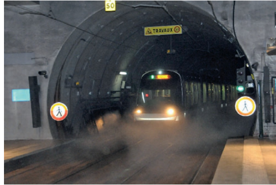
2 Access to an underground station from the hall and introduction of vapor (left-hand image) and moisture to bind particles of railway dust
